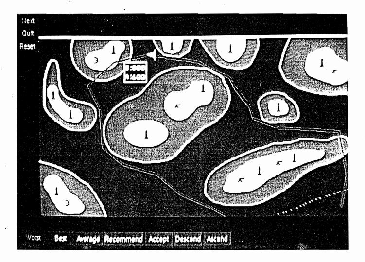
A short while later, the pilot is again illuminated by a surface-to-air threat. The "X" over the yellow arrow indicates that on-board electronic countermeasures have effectively negated this threat.
